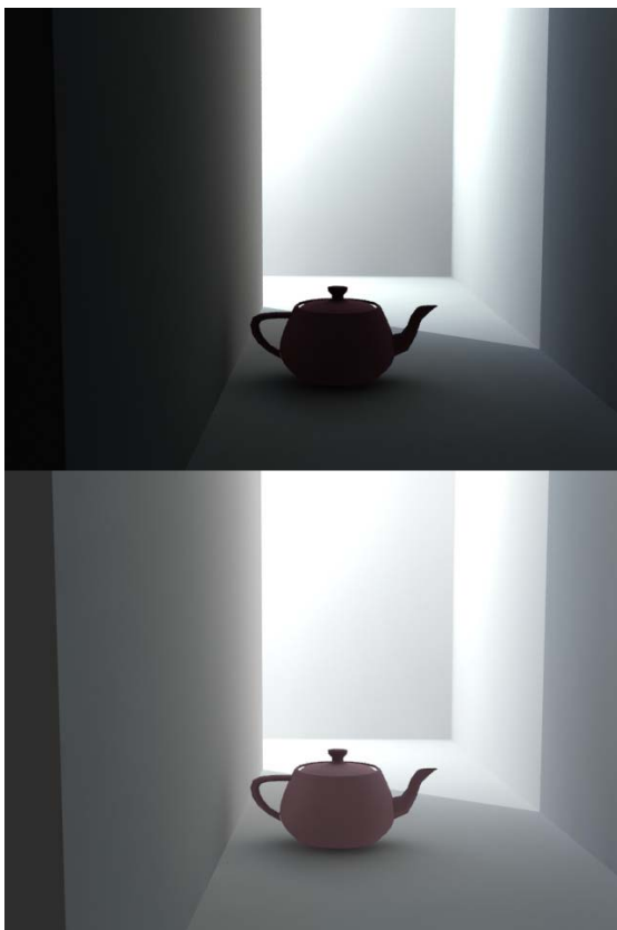
Figure 10 – Example for the influence of gamma correction on global illumination rendering. Top: without, bottom: with gamma correction. Light intensity for the top image was adjusted so the overall brightness of the rear wall roughly matches the one in the bottom image.
